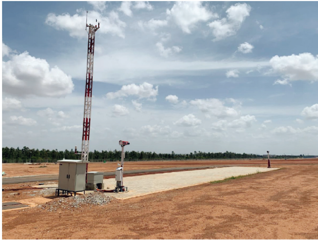
One of the four Dirshts transmissometers installed at the KIA runway to measure Runway Visibility Range (RVR).
