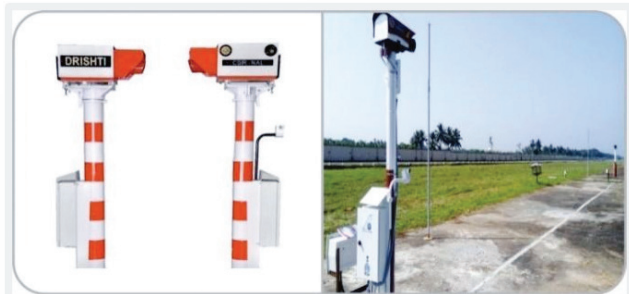
One of the four Dirshts transmissometers installed at the KIA runway to measure Runway Visibility Range (RVR).
