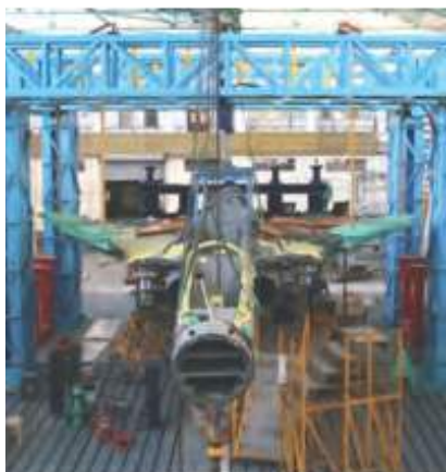
^ Main airframe static test
