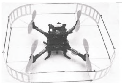
▲ Vision-based auto-pilot system for indoor navigation of MAV
