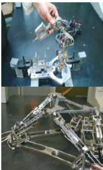
▲ Parallel Kinematic Mechanism (PKM) 6D Robot for neurosurgery
