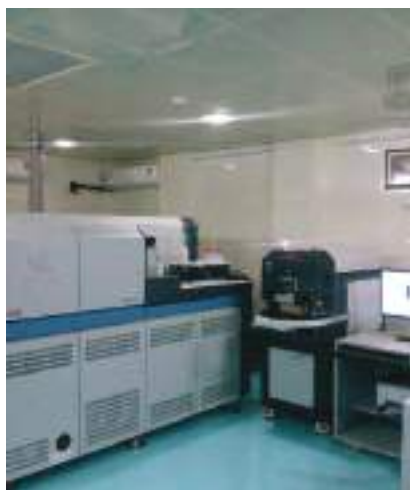
^ Laser Ablation Multi Collector Inductively Coupled Mass Spectrometer (LA-MC-ICP-MS) instrument for isotopic studies
