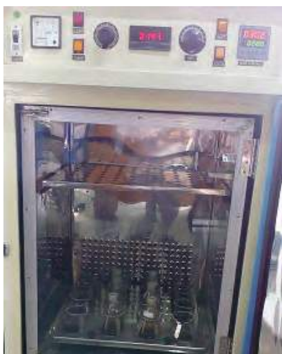
▲ Incubator-cum-orbital shaker with temperature controller and speed controller
