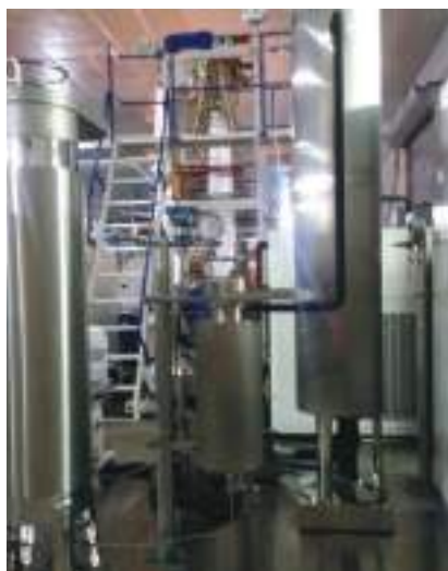
^ Supercritical carbon dioxide set-up for a waterless processing of textiles
