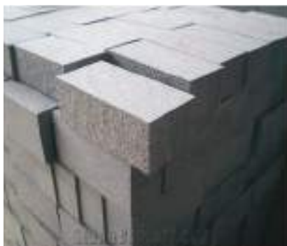
^ Masonry Brick from Granite Sawing Dust
