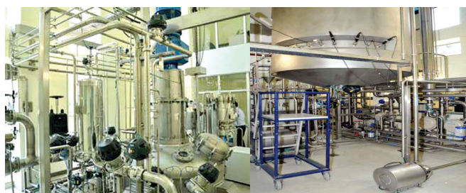
Large-scale production of Oilzapper in 13,000 litre bioreactor
