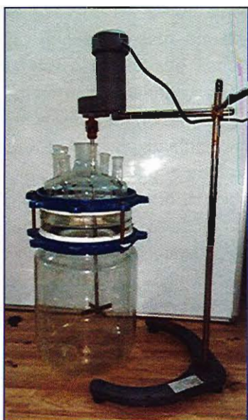
Fig. 23 Laboratory setup for Production of Graphene Oxide
