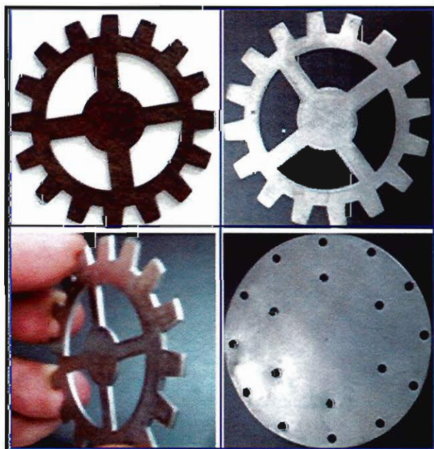
Fig. 29 Electroless RGO-Ni nanocomposite coated components
