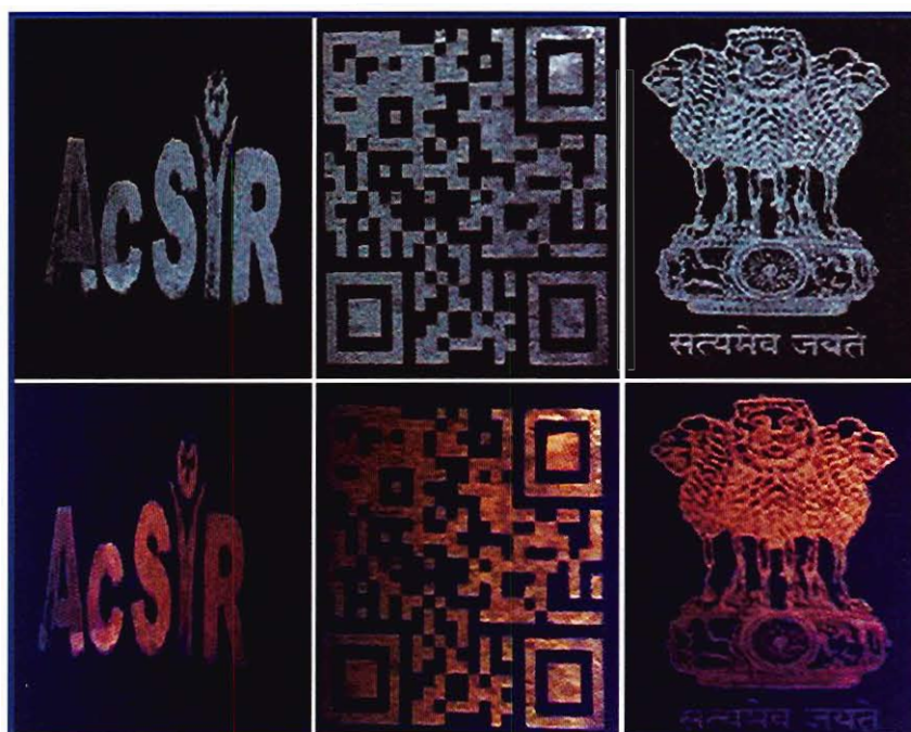
Fig. 49 Prints Using The New Security Ink Appear Differently Under Normal Light (A) And Under UV Light (B)
