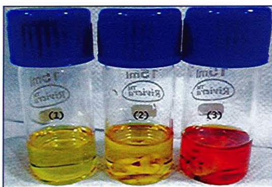
Fig. 24 (1) Sensor solution; (2) Sensor remained silent with non-fluorosis tooth sample; (3) Sensor turns red within 5 minutes of dipping the fluorosis affected tooth sample
