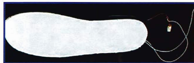
Fig. 44 LTCC/ thick-film hotplate integrated warm-insole
