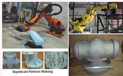
5000 kg single piece stainless steel rapid cast technology
