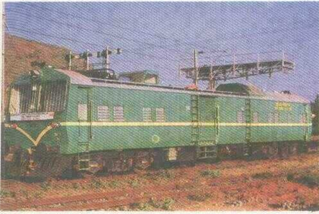
IV.5 OHE Inspection Car.
