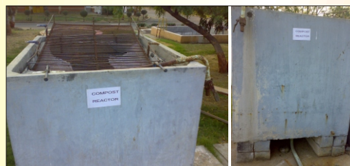
Photograph of pilot plant (Bio- reactor)
