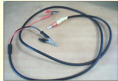
Photo of 10x Probe with Voltage protection for Wave Display 1.0
