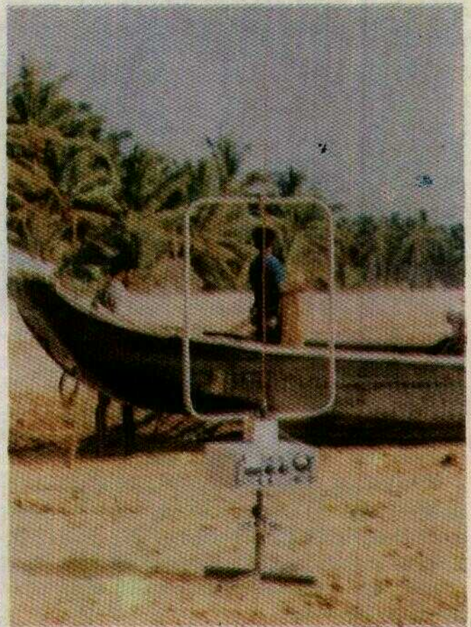
VIII.A.6 Direction finder to locate Radio Distress Signals from fishermen at sea.
