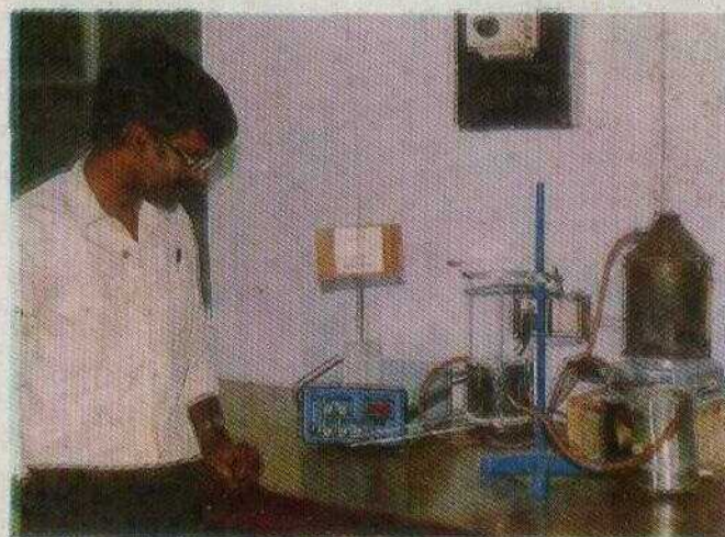
VII.A.1 Thermal Conductivity measurement test for acid proof cement being conducted on Lee's apparatus at IIT Kharagpur.
