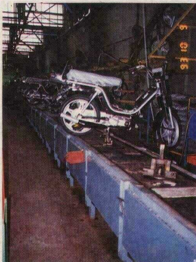
III.C.3. Safari Motorcycle & Assembly Conveyor set up by M/s Kinetic Engineering Ltd., Ahmednagar
