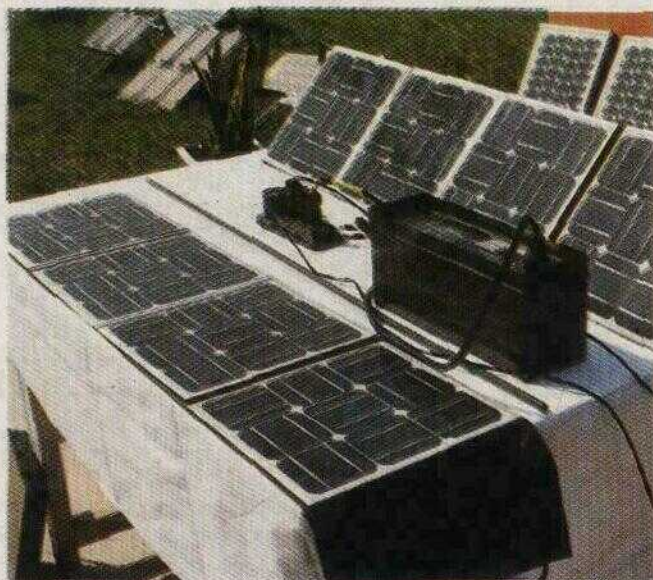
VII.B.1. Foldable Solar Photo voltaic Modules for Charging the Batteries of Man-pack Radio Sets
