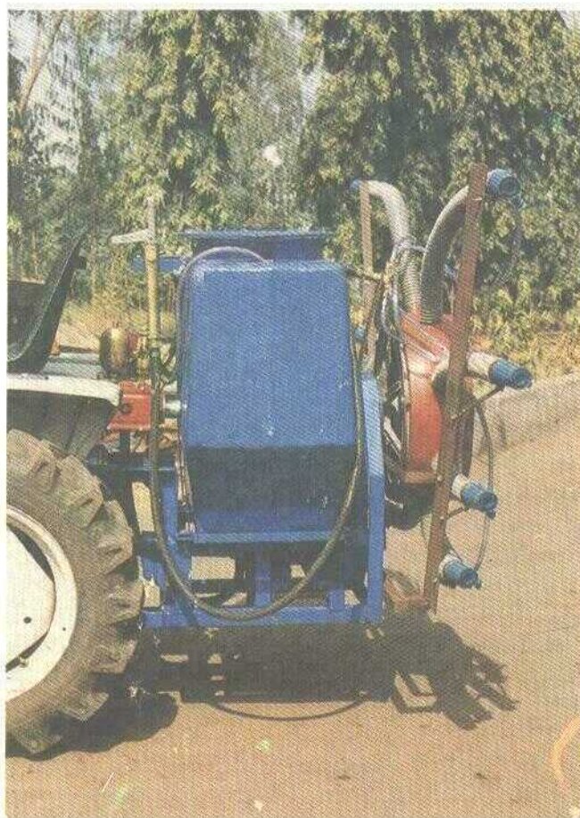
III B.2 Aspee Tractor Mounted Mist blower with Multinozzle Heads for Vegetable Crops
