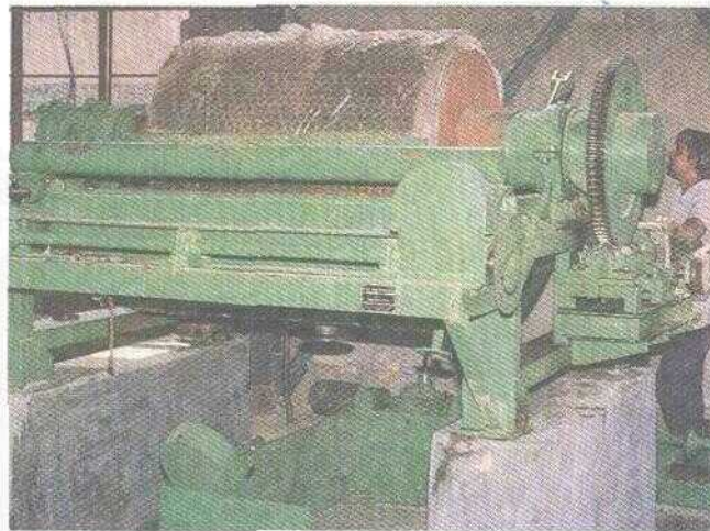
V C.2 M/s Balmer Lawrie's Pilot Plant for Rerefining used lube oil - Rotary Vacuum Filter
