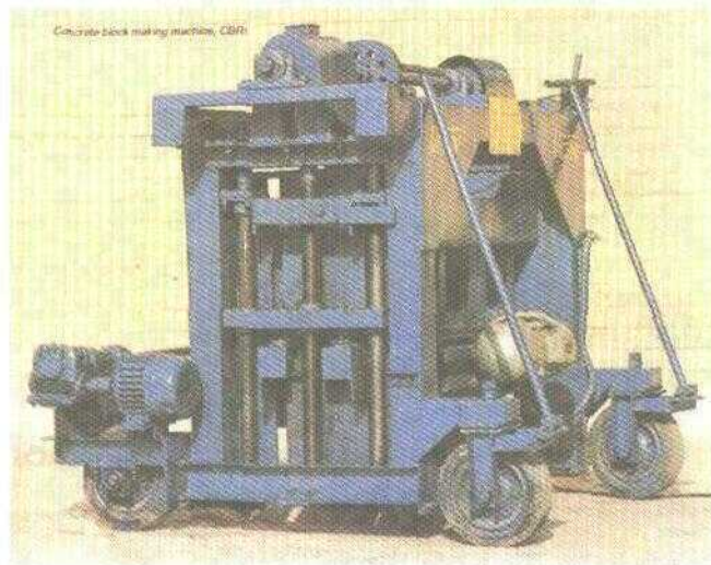
II.6 Concrete Block Making Machine, CBRI
