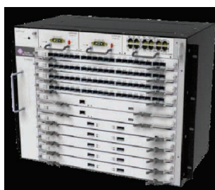
TJ-1600C platform on which the eDC card is hosted to provide eNodeB functionality
