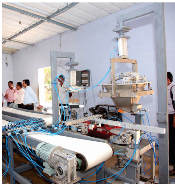
Automated filling system
