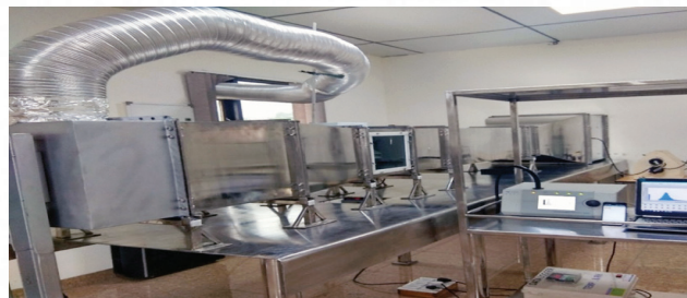
Indigenous developed wind-tunnel facility to test and calibrate PM 1 , PM 2.5 and PM 10 samplers
