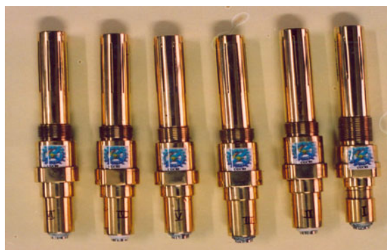
CGCRI developed moisture sensors supplied to P.H. Scientific, UK
