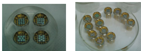
4H-SiC Schottky Diode Detectors ready for delivery
