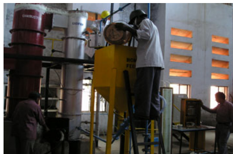
Prototype of entrained flow biomass gasifier system
