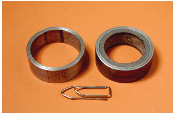
Thermal barrier lining to steel pipe
