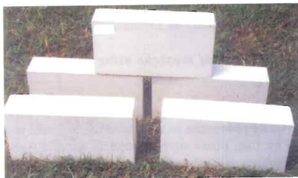
b Gypsum Blocks
