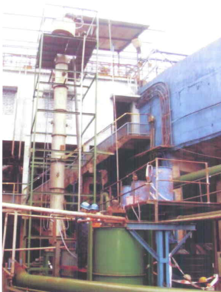
Fig. 37: Column flotation technique for processing of iron ore tailings
