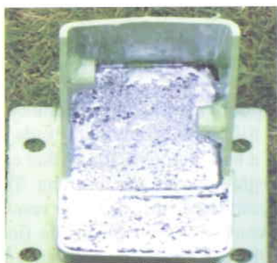
Fig. 39 (a): Foam Filled Crash Box
