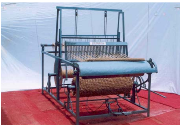
An Improved Mild Steel Handloom for Weaving Matting (An Awarded Invention)
