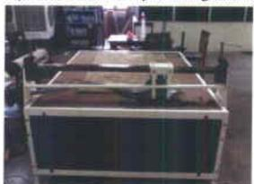
This Carpet Shearing machine may provide less drudgery to artisans and less time for carpet finishing. The machine also provides improved productivity and uniformity in quality, thereby enabling finishing of wool, silk, pashminas and cotton quality carpets. This energy-efficient and eco-friendly machine causes less stress to the workers and can be easily handled. It provides flexibility to finish hand-knotted Tibetan, Nepali and hand tufted type of carpet on the same machine.
