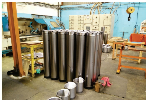
Flow-formed tubes produced at M/s. Paras Flow form Ltd.
