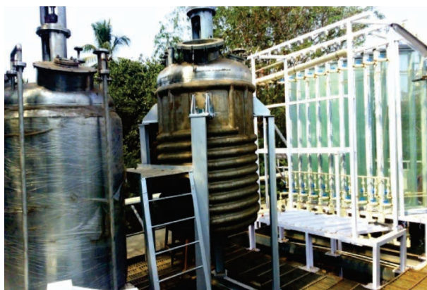
3000L Photo-bioreactor system designed and developed at DBT-ICT Centre for Ulva cultivation
