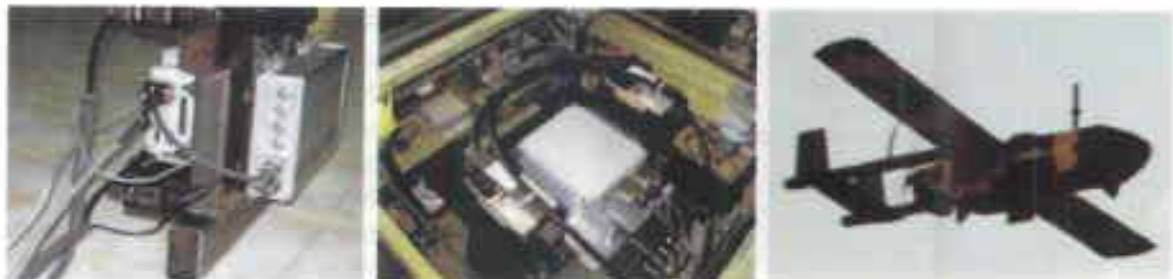
Fig. 1.32. FBG Sensor and SHM system assembled in Nishant UAV; Right, Nishant in flight
