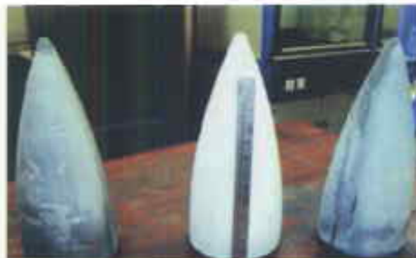
Fig. 1.64. Reaction bonded silicon nitride radomes
