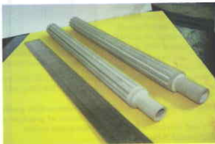
Fig. 1.51. Developed nickel wicks with in-built vapour removal grooves
