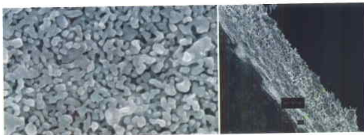
Fig. 1.72. Cross-section of HAp and titania composite layer on Ti metal and the top porous HAp
