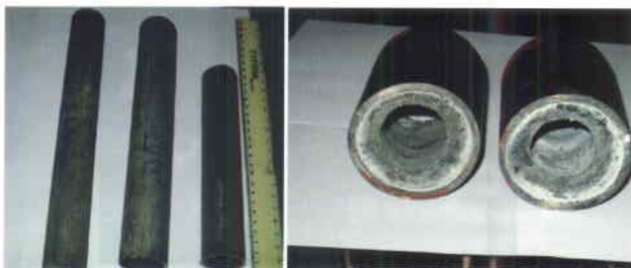
Fig. 1.58. Fe-Al_2O_3 and Al_2O_3-TiB_2 coating inside mild steel and other tube by SHS process
