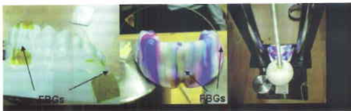
Fig. 1. 87. Jaw Model, Mouth guard and the Experimental Setup
