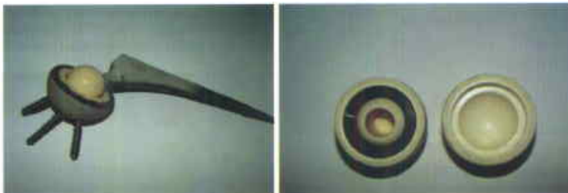
Fig. 1.65. (a) A specimen of implanted all ceramic hip joint prosthesis (b) Bipolar ceramic acetabular cups with ceramic head and bare acetabular cup
