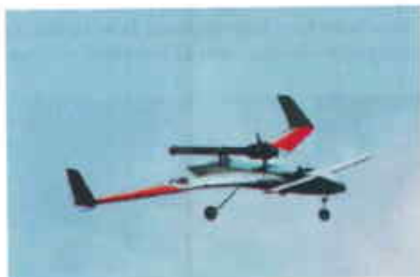
Fig. 1.30. MAV test flight with Pulsejet engine
