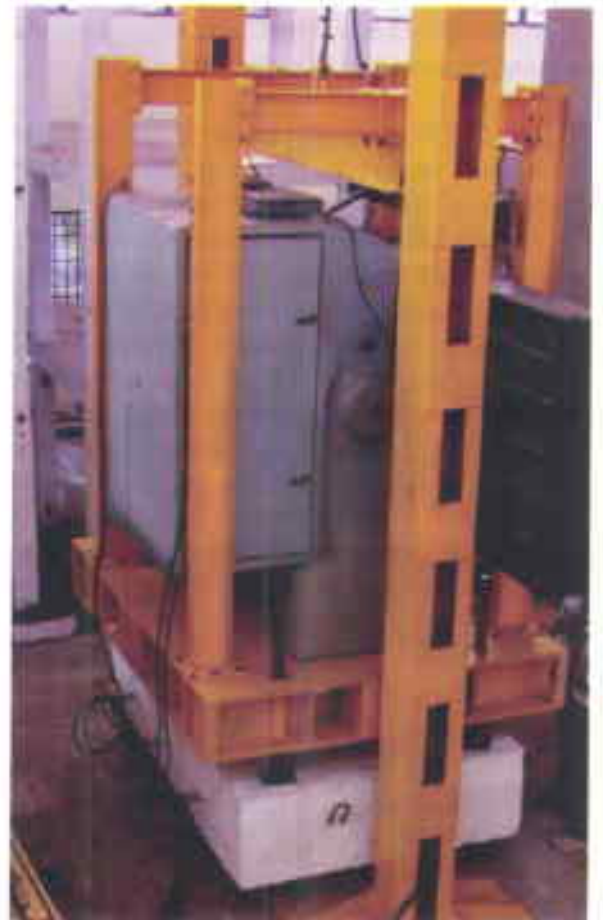
Fig. 1.43. Vertical Shock Test Fixture Layout
