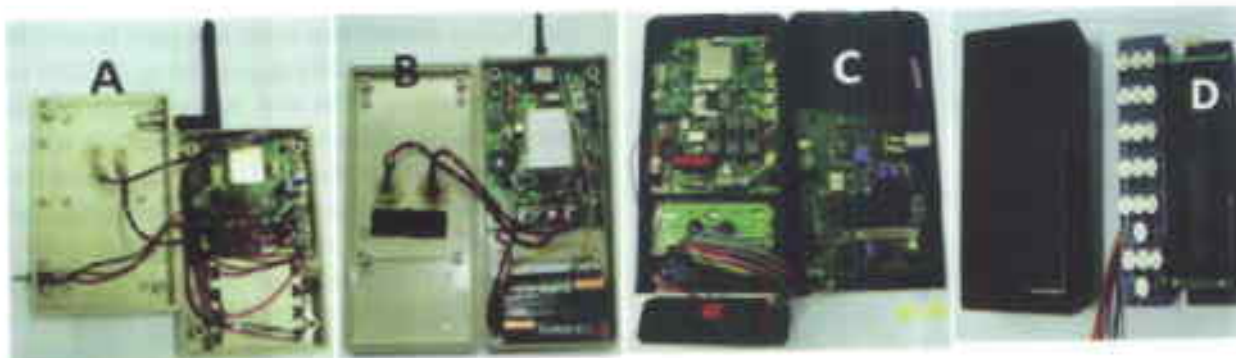
Fig. 1.47. (A) Coordinator; (B) Router/End Device; (C) Gas Monitoring Sensor and (D) Messaging Device with enclosure
