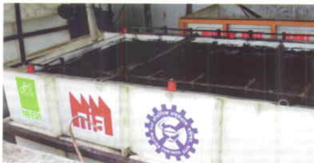
Fig. 1.23. Demonstration of Carbon Bed Electrolyser unit at Nagarjuna Industries, Gujarat
