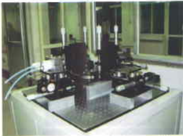
Fig. 1.50. Reconfigurable micro factory test bed
