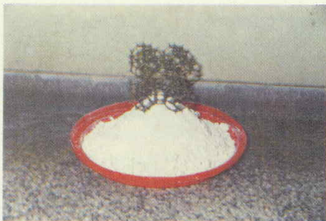
VIII.A.1 Zeolite-A Powder (detergent grade) along with model structure - an awarded invention.
